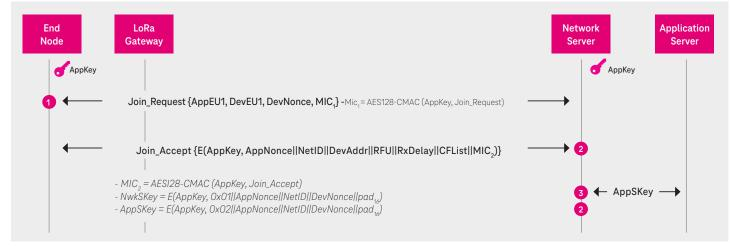
Figure 4: OTAA registration process of a LoRaWAN device [9]
